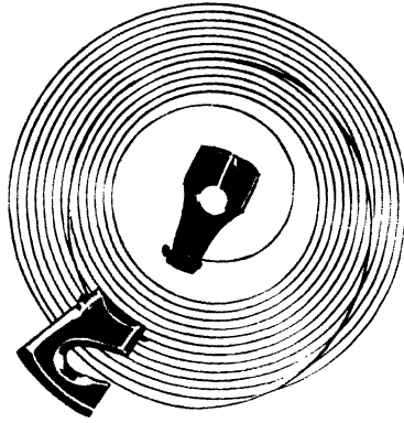
PLATE VII.—The balance-spring of an adjusted watch by Mr. Otto, to which he has applied the inner and outer theoretical terminal.
