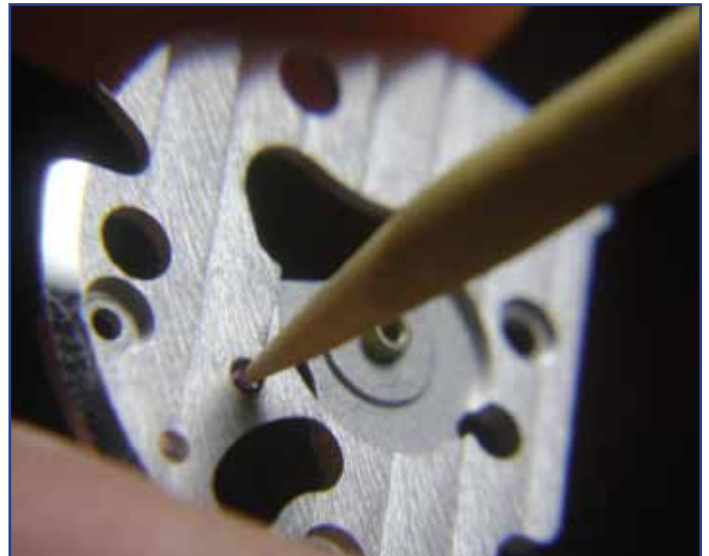
Figure 1: Pegging out a jewel prior to final cleaning to ensure that all traces of previous lubrication that may have dried inside the jewel are removed.
