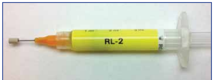
Figure 9: Rolex RL-2 escapement grease eliminates the need for two lubricants.
