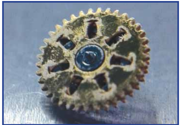
Figure 11: Lubeta V105 leaves behind a waxy film to lubricate reversing wheels.
