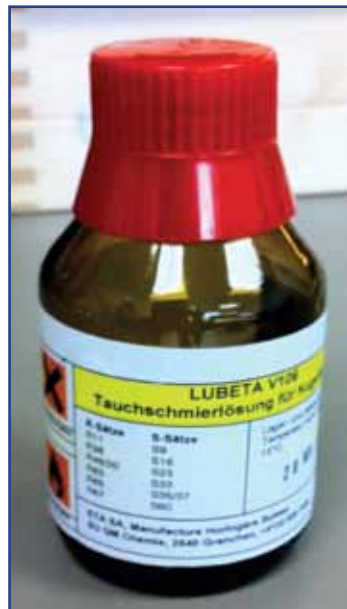
Figure 12: Lubeta V105 and V106 are produced by ETA SA for lubricating specific parts within the watch.
