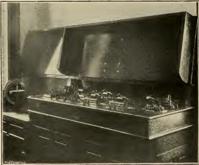
Fig. 4—Instrument Used for Sending Out the Time.
