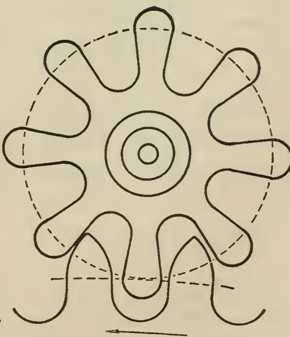
Figure 5. Pinion too small.
