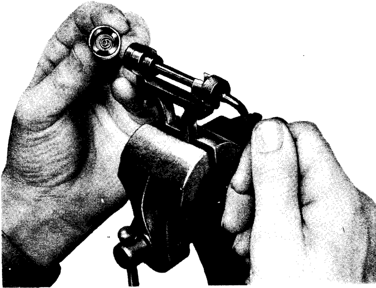
Figure 70 — Mainspring Wound in Barrel
